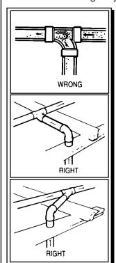
be a pile of dirt at the base of the inlet valve every time it is opened. To avoid this situation the following techniques should be used.
