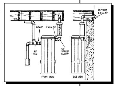
"Vacuums must breath ... do not enclose. If the unit is to be located in a closet or utility room it must be vented. Louvered doors fulfill this purpose. A muffler can, of course, be used to minimize noise.
