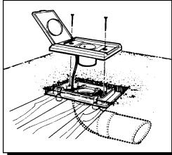
While the normal installation of inlet valves is in partition walls, occasionally one must be installed in the floor. In this case the location for the inlet valve should be about two inches from the wall and not in a high traffic area. As with wall installations use a pilot hole drill to make sure the location is clear of obstructions below. Cut a hole that is 2 1/2" x 4 3/8" in the floor. In the case of linoleum or uncovered floors the mounting plate will be installed from be-
