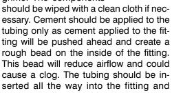
twisted a quarter turn to evenly distribute the cement. All excess cement should be removed with a rag. The glue should be allowed several hours to set before the vacuum system is used.
