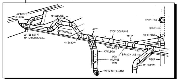
The amount of airflow that reaches the hose is dependent on the efficiency of the layout of the tubing system. Lines are to be kept as straight as possible. Tight 90 degree fittings are to be used only at inlet valve locations and sweep 90 's used in all other applications.
