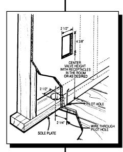
On the floor below apply glue to an adequate length of tubing and aim it upwards through the hole and into the short
