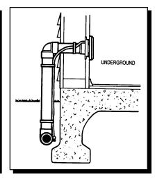
If the tubing is to be buried underground, dig a trench 12 to 18 inches deep along the side of the house. Fully assemble and test the tubing and tow voltage wire before filling in the trench. It is recommended that the low voltage wire installed outside be encased in conduit which is available at most hardware stores.
